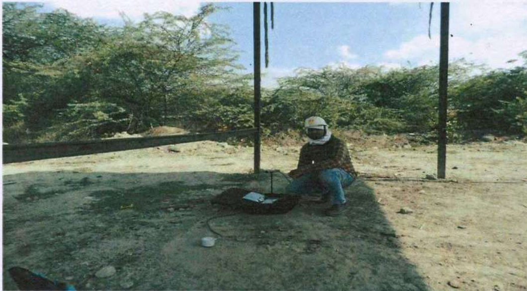
Fig (4 & 5): Setting up of microphone and geophones sensors the measurement of Peak Particle Velocity.
