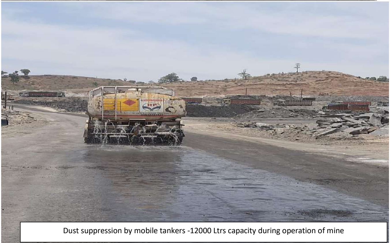
Dust suppression by mobile tankers -12000 Ltrs capacity during operation of mine
